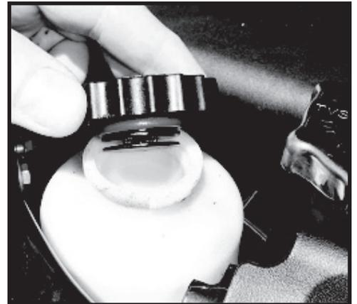
Step 1. Remove the factory power steering reservoir cap by turning counter clockwise. Clean area around cap.
