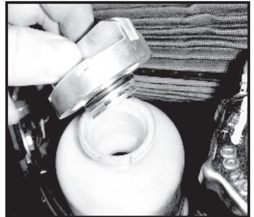
Step 2. Install the new power steering reservoir cap by turning clockwise.
